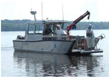
Research vessel Mudpuppy II LOA = 33 ft., B=8.5 ft., D=2.0 ft.
